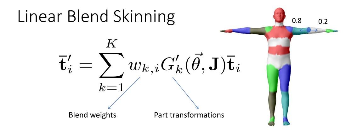
Points transformed as blended linear combination of joint transformation matrices
